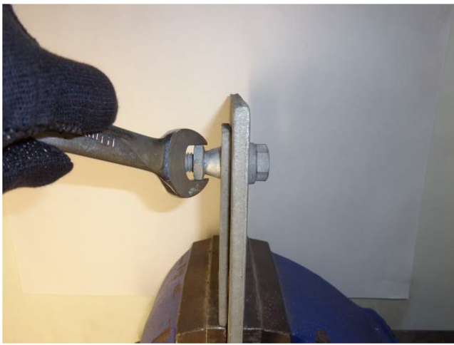
70). Use the spanner and increase tightening.
