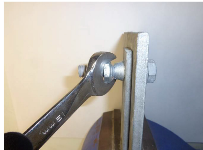
71). Tighten until the nut is broken in two portions.
